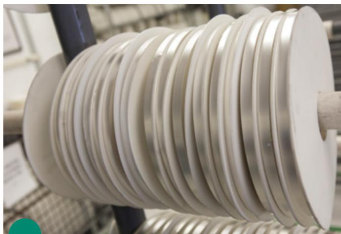
FMC Lithium's Lectro<sup>®</sup> Max line of customized lithium foils is used as the anode in lithium batteries. Lithium, being both the lightest and the most electronegative, provides the highest electrochemical equivalence of all metals.
